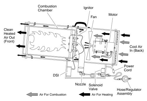
Figure 2 - Cross Section Operational View
